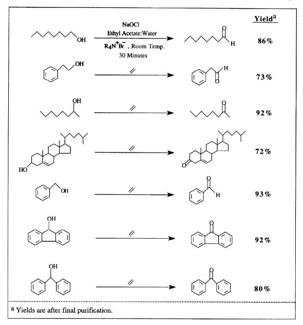
We have shown that phase transfer catalyzed oxidation of primary, secondary, and benzylic alcohols with sodium hypochlorite results in good to excellent yields of the desired oxidized products. This method of oxidation is mild, efficient, and safe. The experimental procedures and work-ups are very convenient. In addition, the low cost and availability of sodium hypochlorite as commercial household bleach makes this method of oxidation of alcohols very attractive.
